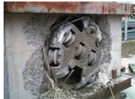
Trial Test Breakthrough at Herrenknecht Factory - Germany
