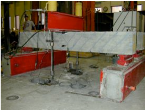
Shear strengthening of concrete beam
