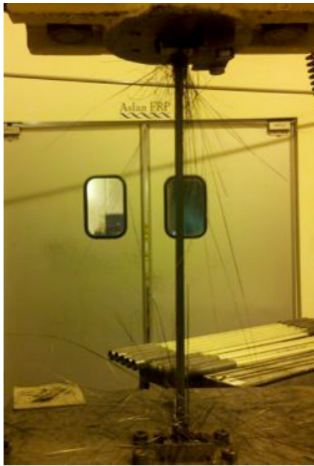
Aslan 400 Laminates with extensometer and after valid tensile test
